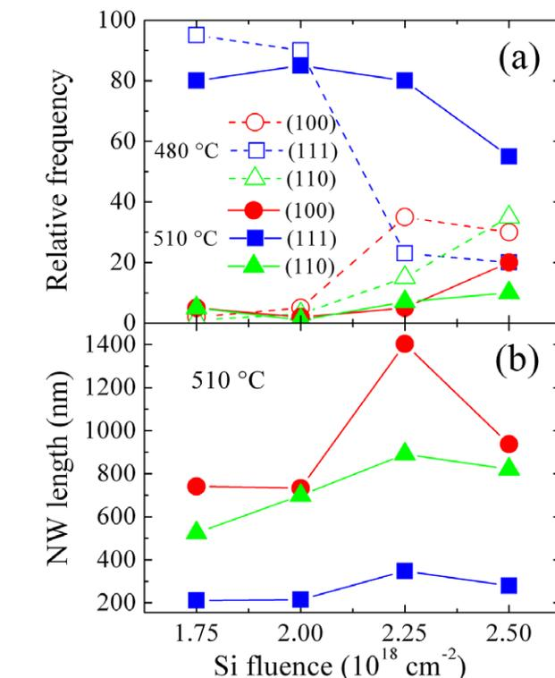
**Figure 5.** (a) Relative population for (111)-, (100)- and (110)-oriented NWs for NWs prepared with a substrate temperature of 480 and 510 °C. (b) NWs mean length as a function of the evaporated silicon fluence for (111)-, (100)- and (110)-oriented NWs grown at 510 °C.
