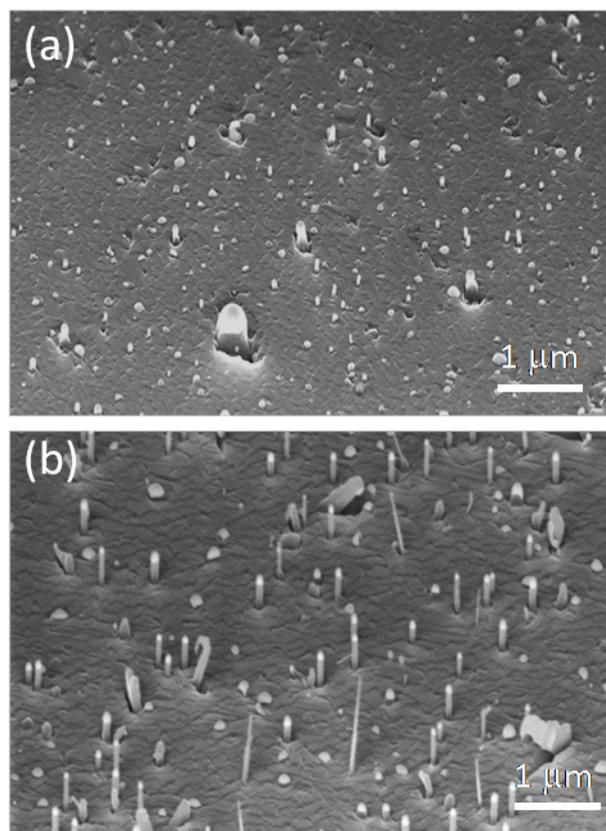
**Figure 2.** SEM images of NWs prepared with a substrate temperature of 480 °C and an evaporated silicon fluence of (a)  $1.75 \times 10^{18}$  atoms  $\text{cm}^{-2}$  and (b)  $2 \times 10^{18}$  atoms  $\text{cm}^{-2}$ .
