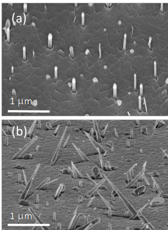
**Figure 4.** SEM images of samples prepared with a substrate temperature of 510 °C and an evaporated silicon fluence of (a)  $2.0 \times 10^{18}$  atoms  $\text{cm}^{-2}$  and (b)  $2.50 \times 10^{18}$  atoms  $\text{cm}^{-2}$ .
