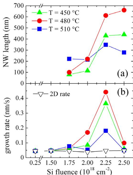
**Figure 3.** (a) Measured mean length of (111)-oriented NWs for samples grown at different temperatures. (b) 2D and axial rate values as a function of the evaporated silicon fluence for (111)-oriented NWs grown with substrate temperatures of 450, 480 and  $510^\circ\text{C}$ .
