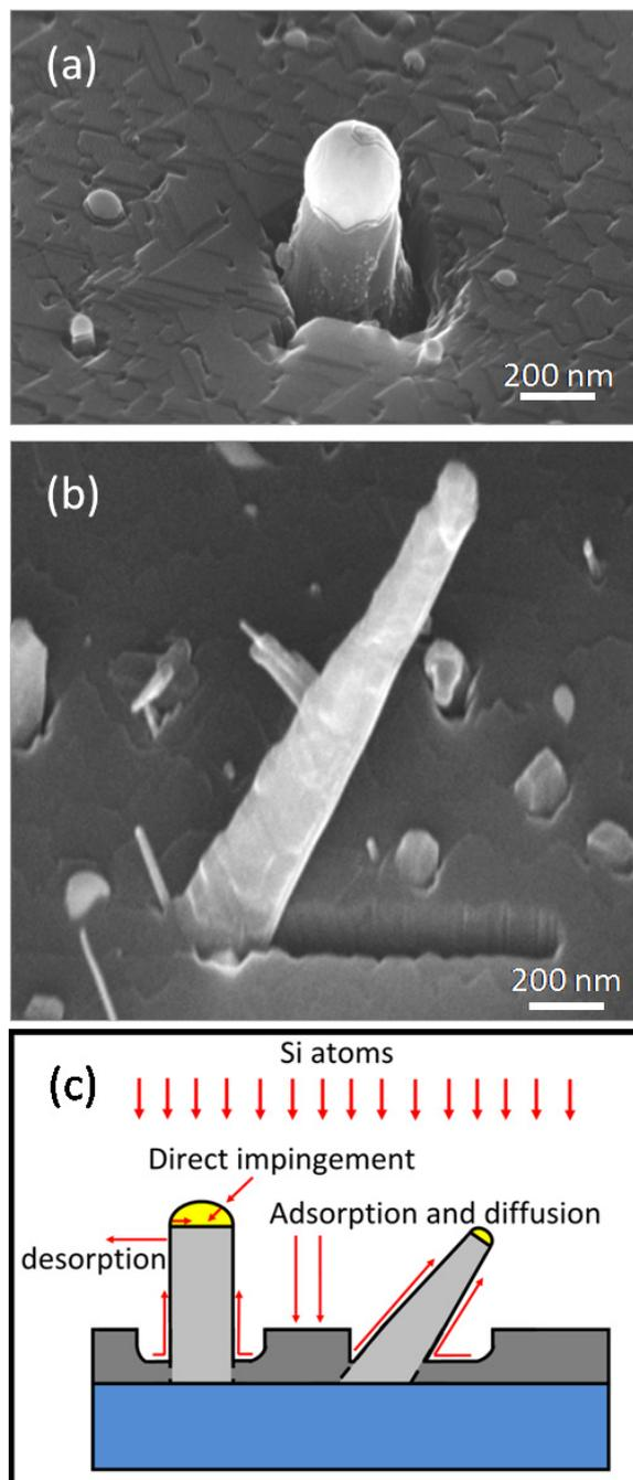
**Figure 1.** (a) SEM images of a cylindrical (111)-oriented well-shaped NW and (b) of an inclined (100)-oriented NW. Note in both cases the gold droplet on the top and the dip at the base. (c) Scheme of the proposed model for Si NW growth by EBE.
