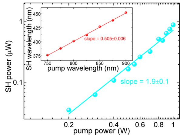
FIG. 2. Pump power dependence (log scale) of the emission peaked at 375 nm (750 nm excitation wavelength) from as-deposited silicon nitride with 46.2 at. % Si content. The continuous line is the best fit of the experimental data. (Inset) Measured second harmonic wavelength as a function of the excitation wavelength for the same sample. The continuous line is the linear fit of the experimental data.
