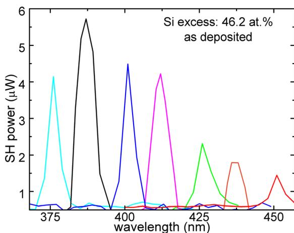
FIG. 1. Second harmonic spectra from as-deposited 46.2 at. % Si content silicon nitride after pumping with excitation wavelengths between 750 and 900 nm. All data have been taken at the same pumping power (1 W).
