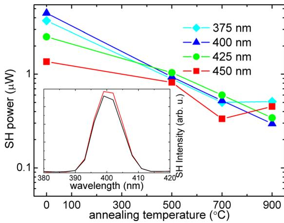
FIG. 4. Second harmonic power detected after pumping with different excitation wavelengths with the same pumping power as a function of the annealing temperature for the sample with 46.2 at. % Si content. (Inset) SH spectra for the as grown sample, with (black line) and without (red line) a 30 nm-thick SiO<sub>2</sub> cap layer.
