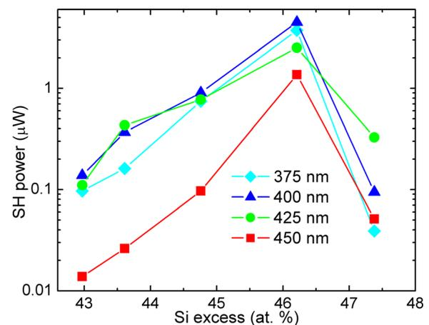
FIG. 3. Second harmonic power detected after pumping with different excitation wavelengths with the same pumping power as a function of the Si content.
