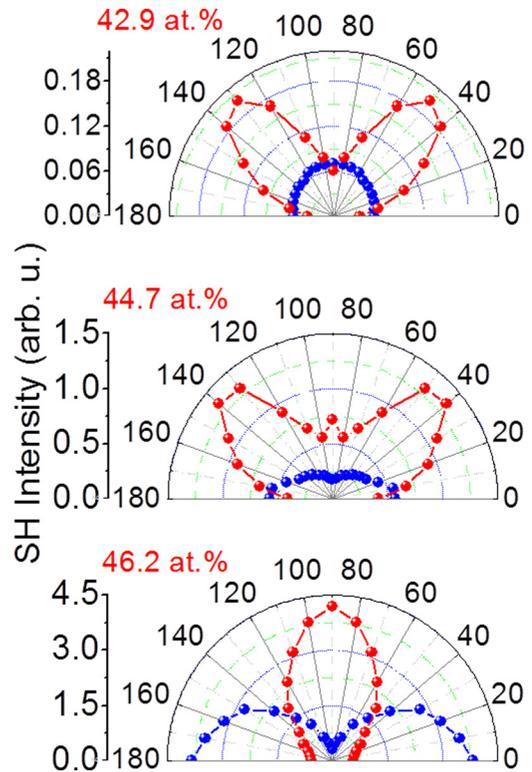
FIG. 5. Polar plots of the second harmonic intensity (arbitrary units) generated at a pumping wavelength of 800 nm in samples with different Si content, as-deposited. The pump polarization is changed and the detection polarization fixed at the s (red dots) and p (blue circles) polarization components.  $0^\circ$  corresponds to p-polarized pumping light;  $90^\circ$  to s-polarized pump.
